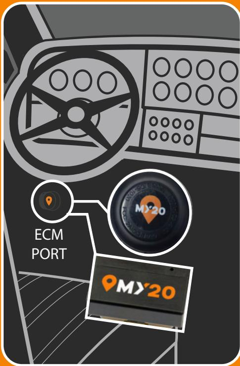
To install the MY20 ELD, match the pin configuration on the back of the ELD to your ECM connector (9pin or OBDII). Once the center pin "key" is aligned in the "slot", push the device to fully seat it, and then turn the outer locking ring clockwise (to the right) by 1/8 of a turn to lock it in place
