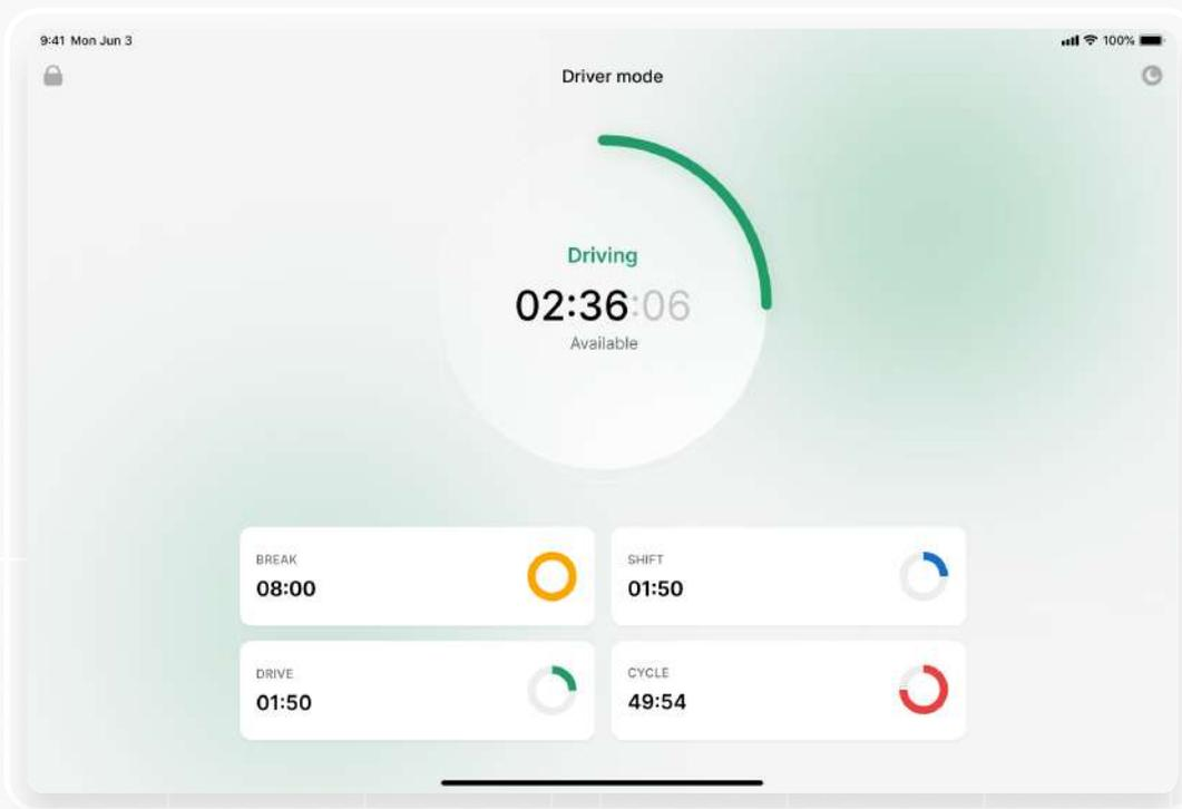
Once you have connected your mobile device to NEW, your driving time automatically recorded. When your vehicle begins moving, your duty status will automatically be set to **Driving**. At 5 mph (or more) the vehicle is considered **Drive**.
