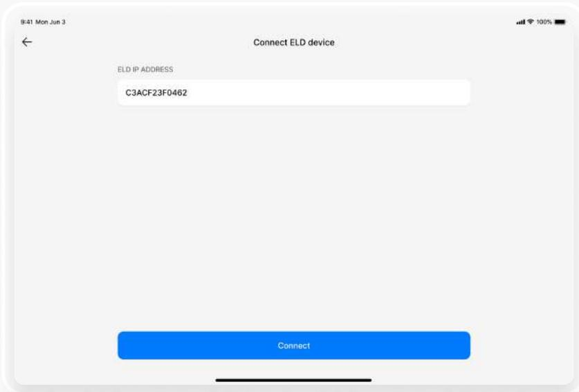
By touching on the screen of mobile device application can get IP Adress of the ELD. By pressing '**Connect**' button ELD device starts working with our application.
