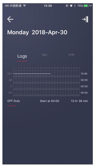
You can see 24-hour Duty Status Grid and the details of the data. In addition, there are two other functions namely "Sign" and "DVIR" in this page.
