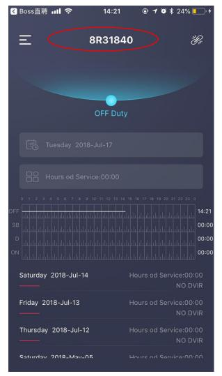
The license number of the selected vehicle is shown on top of the Home page (marked by a red circle here). The system starts to record automatically your Hours of Service and Duty Status.
