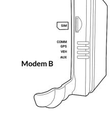
On Modem B, an active GPS location and server connection is ON when the GPS light is a solid green and the COMM light is a solid orange.
