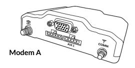
On Modem A, an active GPS location and server connection is ON when the GPS light is a solid green and the COMM light is a solid orange.
