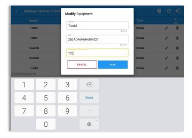
An **Odometer Offset** allows driver or personnel to adjust the odometer so that the driver will see an odometer matches their dashboard, rather the engine odometer. Possible scenario is when the engine is replaced and the value is not yet synchronized.
