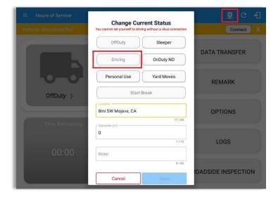
A *Requires VBUS connection for driving* option prevents drivers from changing to Driving status if they are not connected to a VBUS device. Drivers must have their tablet, iPad, or mobile device connected with the VBUS device using a tethered, Bluetooth, or WIFI-direct connection.
