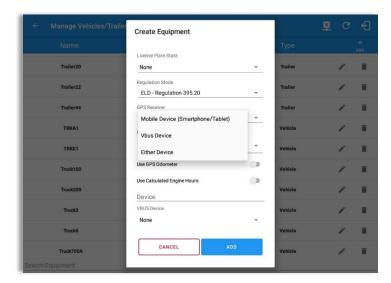
A **GPS Receiver** option allows the user to change how to get the device GPS positions. The GPS Receiver settings can be set in a specific vehicle in the portal->equipment management page.
