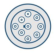
9-Pin J1939 Port In most heavy duty vehicles later than 2005
