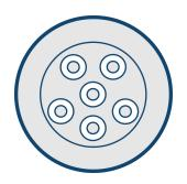
6-Pin J1708 Port In most heavy duty vehicles manufactured before 2006
