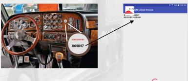
On the ELD, select the ECM-linked device's ID showing on the dashboard's decal (if vehicle equipped with decal).
