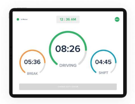
Once you have connected your mobile device to EVO ELD ELD, your driving time automatically recorded. When your vehicle begins moving, your duty status will automatically be set to "**Driving**". At 5 mph (or more) the vehicle is considered to "**Drive**" and "**On Duty**"
