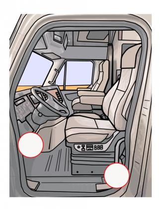
4. Now that the diagnostic port has been located attach the cord to the ELD Hardware (if you have the black box or OBD2 Connection Cord is needed) — next attach the cord to the diagnostic port – Confirm the set up of the on arrangements as you will need to contact support if the chord does not match the correct pinout. (6 Pin, 9 Pin, OBDII)
