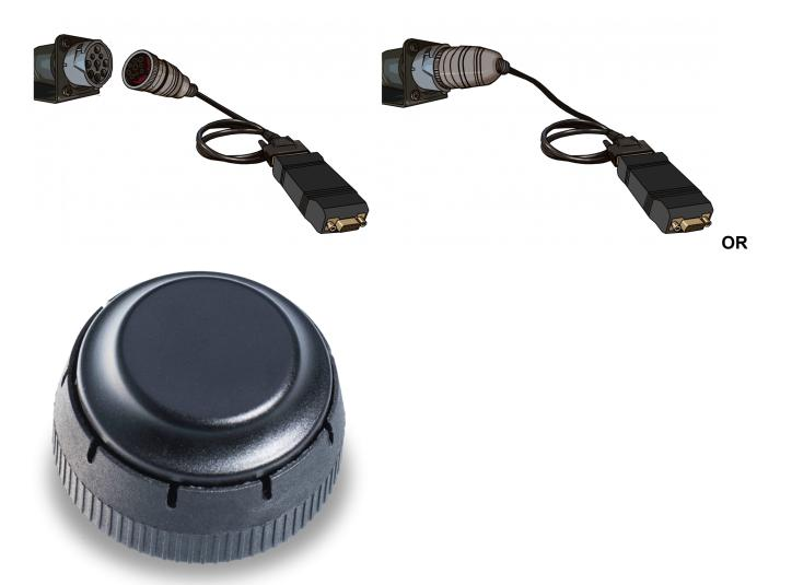
5. • Once connection is made if applicable run wire to top of the dash and place tape and secure device to the stop of the dash – if unit is plugged on the floor outlet secure ELD device via tape to the sidewall of the cabin (Not Necessary for Circle ELD devices)
