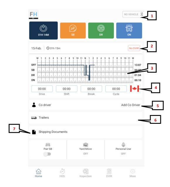
1. <u>Bluetooth Connection</u> — Used for connecting the app with the ELD.
