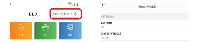
2. Upon selecting the vehicle, the Bluetooth connection will be established, and the vehicle icon will turn Blue. As shown below.
