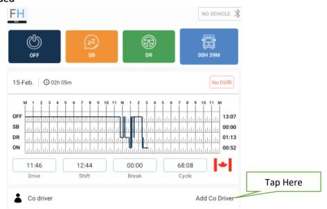
2. For switching the co drivers, click on the co driver name and select driver under "Switch Driver".
