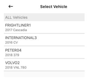
4. Tap on the ELD icon on the top right corner of your screen. If there's a currently selected vehicle then select 'Leave vehicle'. Go to your device's Bluetooth settings and reset the Bluetooth connection by turning it off and then turning it back on. Now, reselect the vehicle you want to connect to. The connection dialog box should appear and connect the ELD to your app. If this step doesn't resolve the connection issue, then follow step 3.
