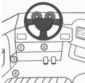
3. Insert ROAD STAR ELD device into the diagnostic port of the vehicle.
