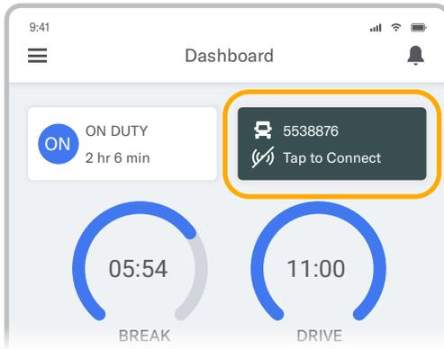
1. Use Tap to Connect bar to connect to your vehicle. The device will attempt to connect to selected vehicle ELD via Bluetooth. ELD bar will change from red to orange: Pairing.
