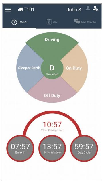
When the truck is stopped for more than 5 minutes, the driver will be prompted to select their duty status and will have 1 minute to respond. If the driver did not respond the duty status will be automatically set to *On-Duty Not Driving*.
