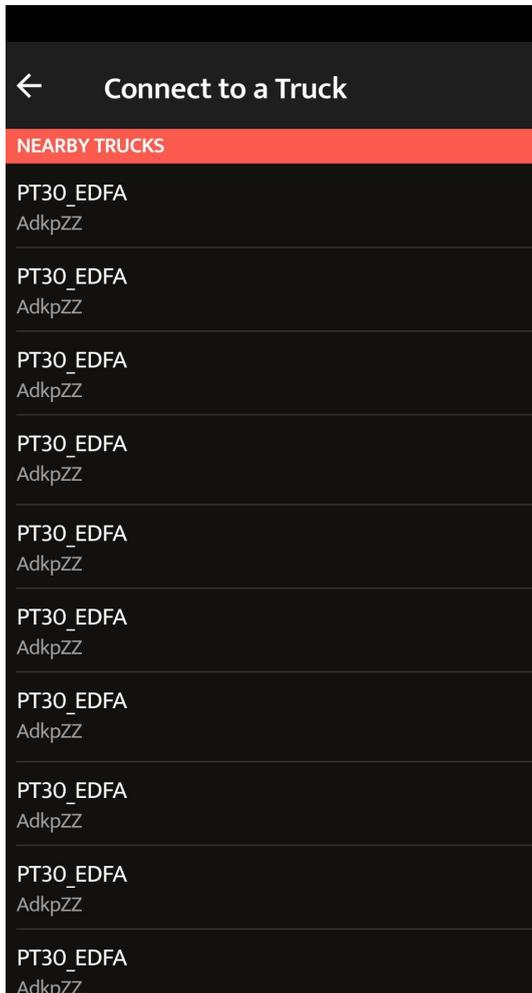
Once you have connected your ELD device to your vehicle, it's time to set up a connection with the Pro-Tracking application. To do so, you need to turn on the Bluetooth on your smartphone or laptop and enter the app. After that click the Truck icon at the top of the app's Main screen. The app will scan all the nearby trucks for the ELD presence. Select your truck and ELD by the serial number from the list and start using the app.
