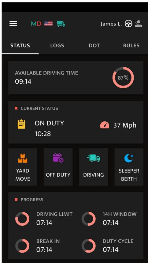
Please use the Switch Status interface to change your current status to another one. The Driving status is recorded automatically by the ELD within 3-10 seconds after the start or stop of a vehicle's engine. In case you need to switch the status, you should stop, wait till the Switch Status interface becomes clickable and make changes after that.
