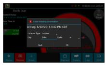
**Tip:** If the logging device frequently prompts you to enter location data, check the GPS antenna to ensure that it is not loose or disconnected.
