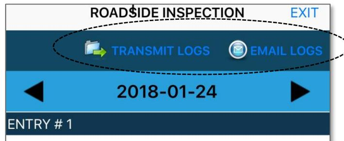
*Option 1:* To share the Roadside Inspection report via FMCSA Web Services, **Select** the **Transmit Logs** (refer to Figure 9.), and your Roadside Inspection Report will be transferred to the FMCSA web server.
