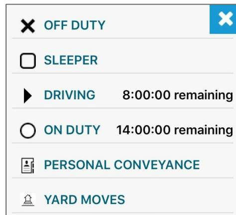
Changing the status in some instances, will prompt the driver to add optional comment. Additionally, status will be automatically changed to Driving, or On Duty, based on the ELD input from the engine.
