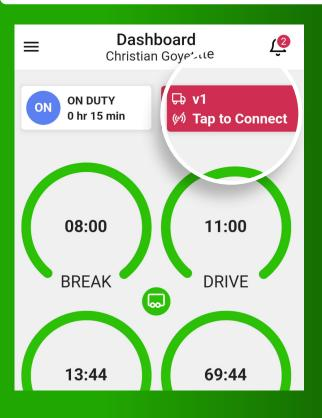
Use **Tap to Connect** bar to connect to your vehicle. The device will attempt to connect to selected vehicle ELD via Bluetooth. ELD bar will change from red to orange: **Pairing**
