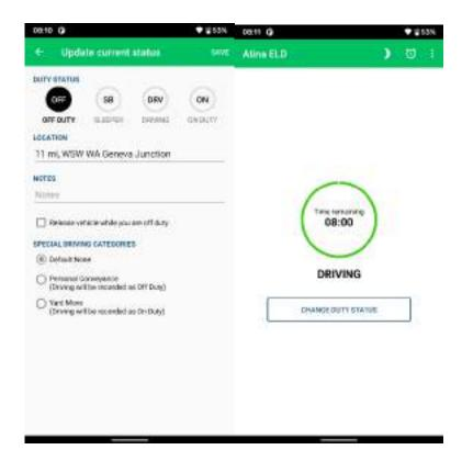
When the ATINA TECHNOLOGY gateway is able to obtain a valid GPS fix, the Location field will be automatically populated with the current location information of the user. If there is no GPS fix, the Location field will remain blank, in this instance and you must manually input the relevant details.
