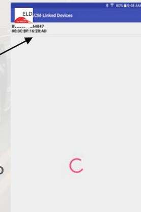
On the ELD, select the ECM-linked device’s ID showing on the dashboard’s decal (if vehicle equipped with decal).
