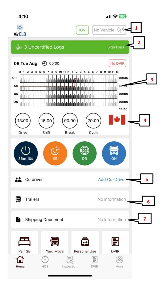
1. Bluetooth Connection — Used for connecting the app with the ELD.
