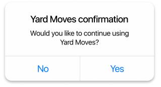
For drivers within Canadian operating zones, the Yard Moves option will also be automatically reset to "**Off**" when the vehicle's speed exceeds 32 km/h.
