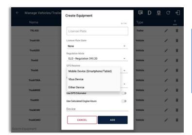
A **GPS Receiver** option allows the user to change how to get the device GPS positions. The GPS Receiver settings can be set in a specific vehicle in the portal->equipment management page.
