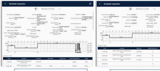
Roadside Inspection screen for vehicle in **ELD** mode
