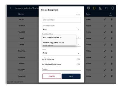
A *Regulation Mode* option to switch between 395.15 (AOBRD) and 395.20 (ELD) support is available. When 395.15 (AOBRD) mode is selected it turns off all 395.20 (ELD) features. It simply records the drivers' events regardless to the FMCSA rules. ELD is set as the default regulation mode for all new equipment.
