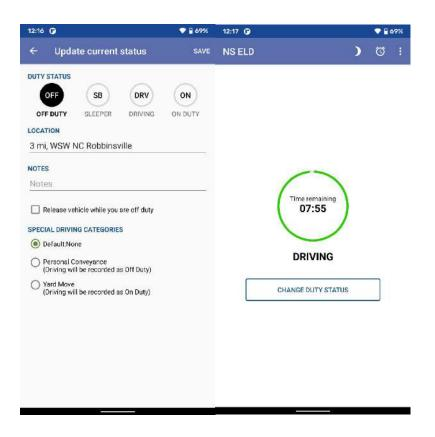
When the NS ELD gateway is able to obtain a valid GPS fix, the Location field will be automatically populated with the current location information of the user. If there is no GPS fix, the Location field will remain blank, in this instance and you must manually input the relevant details.
