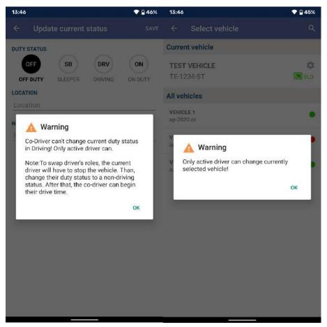
Note: Only active driver can change his duty status to Driving. If Co-Driver tries to do this, warning dialog opens. The current driver will have to stop the vehicle and change their duty status to a non-driving status before the co-driver can begin their drive time. Also, Co-Driver can't change active vehicle or release it. Only active driver can do this.
