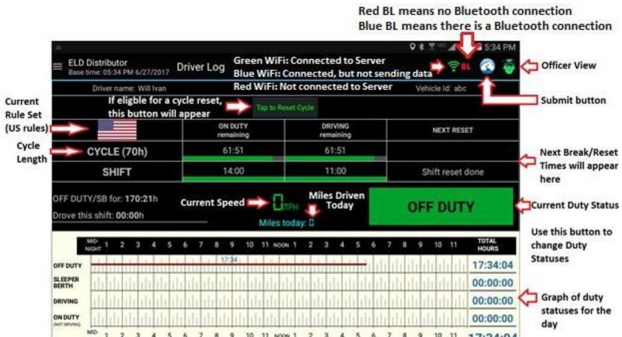
**NOTE: Officer with a Green face means no diagnostic errors, Orange means at least one diagnostic error, and Red means at least one malfunction.**
