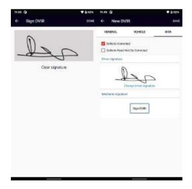
When you return to the main DVIR tab, on the selected Log, the inspection report that you have created will be shown. Also, on the main Logs screen, the Wrench icon will reflect the changes made, i.e. if you have reported 2 defects, it will change from No DVIR to 2 Defects.
