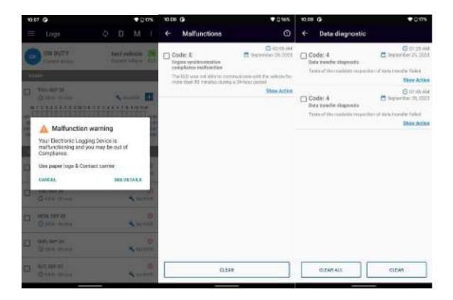
When you see the malfunction indicator, you should view the malfunction details by tapping the indicator. This opens the 'Malfunctions' screen that lists malfunction events recorded on the ELD. You can view the details of a malfunction and clear it.
