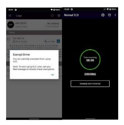
When the Nomad ELD gateway is able to obtain a valid GPS fix, the Location field will be automatically populated with the current location information of the user. If there is no GPS fix, the Location field will remain blank, in this instance and you must manually input the relevant details.
