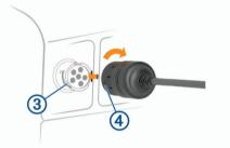
5 Turn the lock ring clockwise until it locks into the vehicle port.
