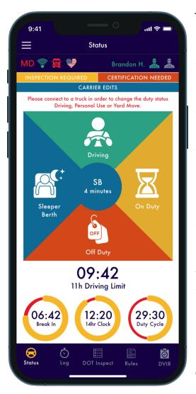
The "Driving" status is automatically recorded within 10-15 seconds after the vehicle begins moving. When driving concludes, it's important to stop and wait for up to 20 seconds until the ELD device acknowledges the end of the Driving event. Only then should you proceed to turn off the engine.
