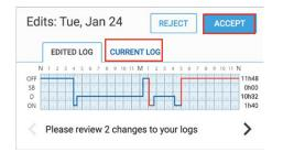
3 Tap the **Accept** ACCEPT button if you agree with the change or tap the **Reject** REJECT button. The Carrier Edits screen displays a confirmation message when completed. An accepted change updates your log, and you have to recertify any affected days.
