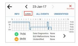
4 Tap the **Right** → arrow to see driver status changes in the log or tap the **Left** < arrow to return to the first (Logs) tab screen. The inspector can see details for each duty status.
