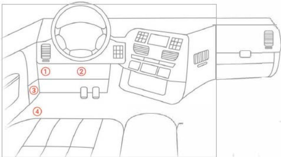
1. With the engine off, locate the diagnostic port inside the vehicle. The diagnostic port is generally located in one of four places:
