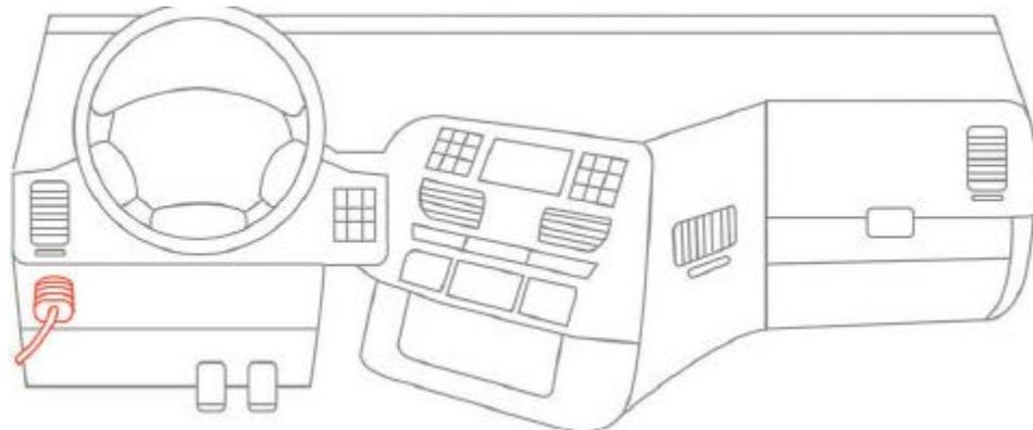
2. Attach the 9-pin, 6-pin or OBDII cable and device to the diagnostic port of the vehicle.
