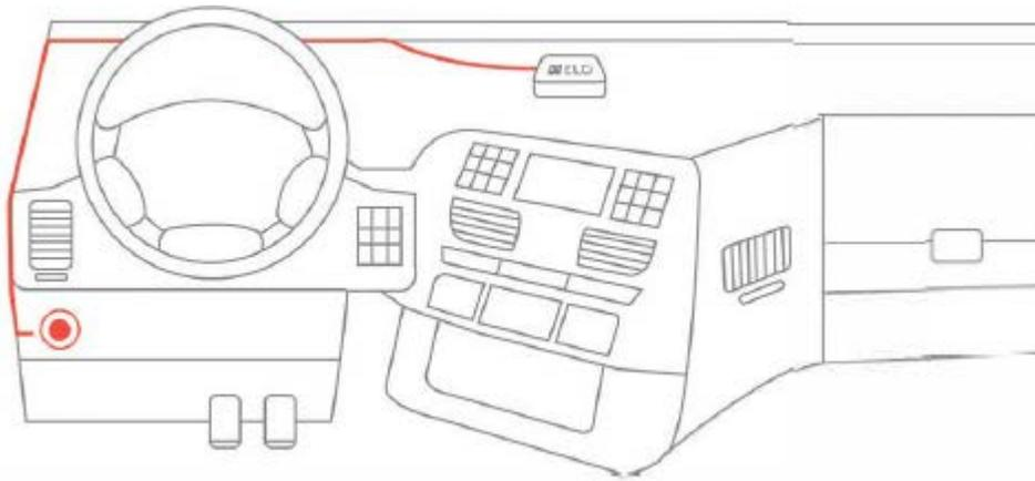
4. Choose a spot on the top of the dashboard to mount your ELD. The mounting spot should be near the windshield, but away from any vents or electrical components that may cause interference.
