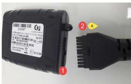
Plug the cable at the of the harness **2** **A** into the ELD device **1**
