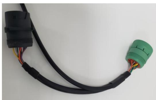
With the engine off, plug the long cable into the vehicle's diagnostic port. This is usually located under the left side of the dashboard or driver's left kick panel.
