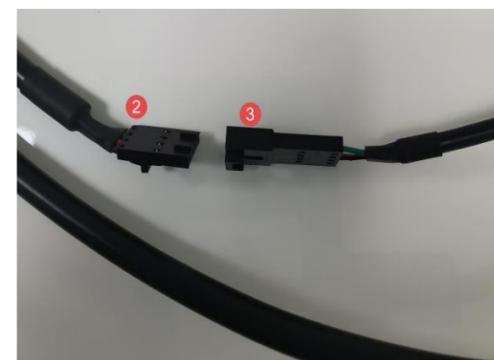
Plug the BT Extender **3** into the short cable of the harness **2** **D**
