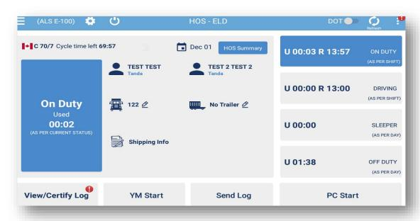
The User Interface is kept very simple so that it will be very easy for driver to use. In order to change any statuses driver just need to click on any one of thefive buttons. Upon clicking the button it will automatically update the statuses of the driver and also calculate the number of hours used and remaining.
