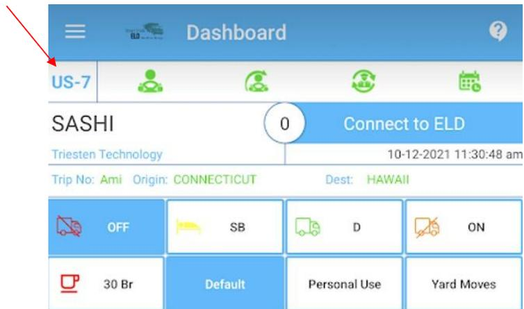
Your Driver Duty Limitation status is located in the top left most icon, which reflects the type of driving you selected from the website for that particular driver. There are currently 12 types of driving limitations. You can switch to Canada rule from default rule by using switch option from Settings on the left side menu.
