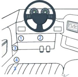
2. Attach the device to the diagnostic port of the vehicle.
