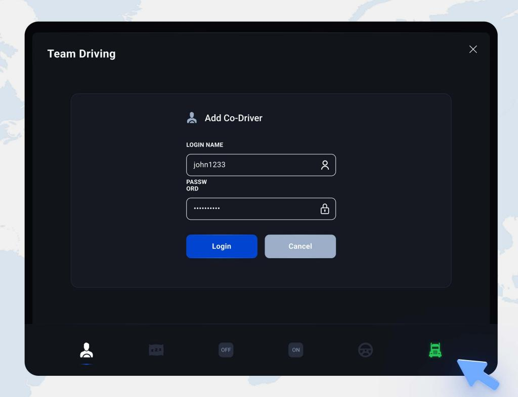
If the ELD is connected to vehicle driver can see green icon on the right side of dashboard. Optional Team driving by adding Co-Driver using credentials.
