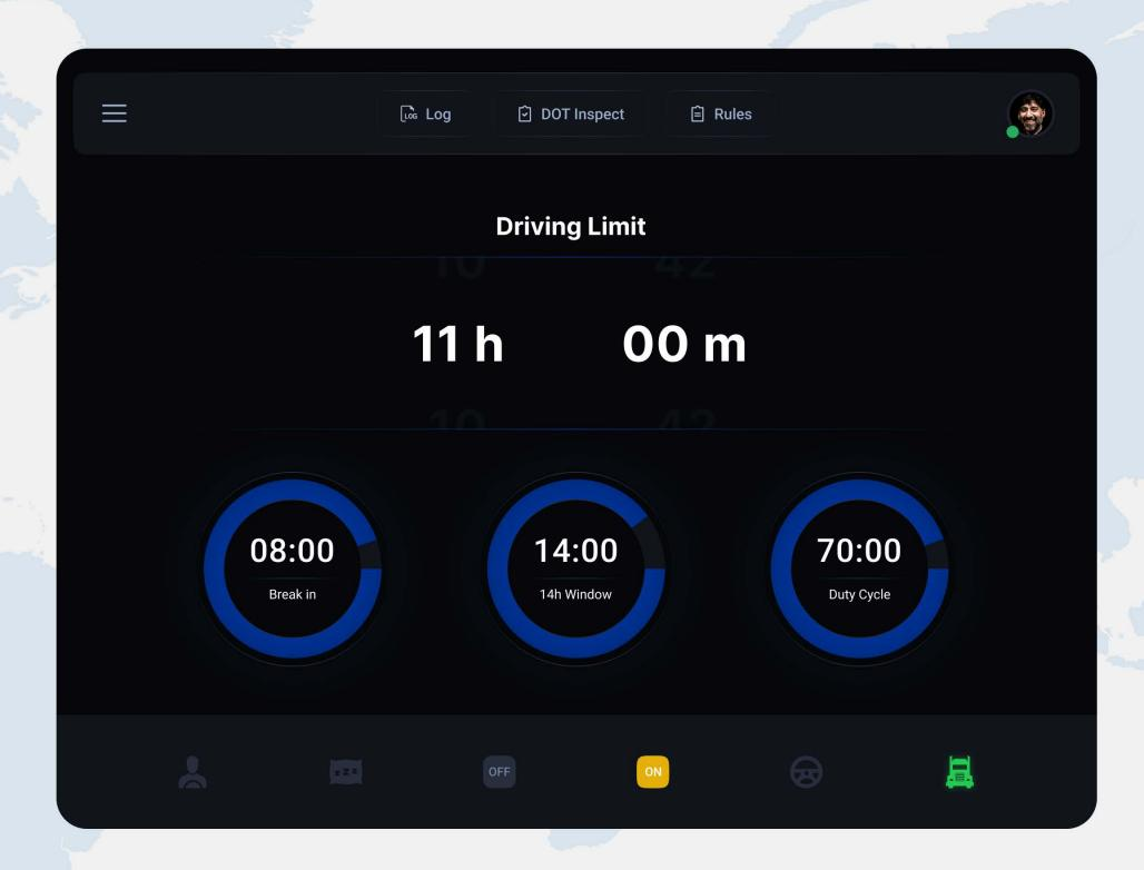
Your driving time automatically recorded. When vehicle begins moving, duty status will automatically be set to "Driving". At 5 mph (or more) the vehicle is considered to "Driving" and "On Duty".
