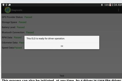
This process can also be initiated, at any time, by a driver in case the driver switches trucks or a Diagnostic/Malfunction indicator turns red (go to the Menu and select Diagnostic).
