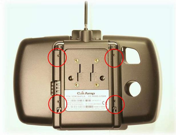
Optional: to securely mount the tablet to the dock, dock the tablet and insert the Tablet Docking Screws into the MDT7 V-Series dock.
