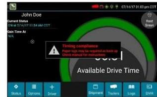
You must document the occurrence of a compliance malfunction and notify your carrier in writing within 24 hours and reconstruct your record of duty status for the current 24-hour period on a paper log. If the malfunction prevents you from accessing your logs on the device, you must reconstruct your previous 7 consecutive days of logs on paper as well.
