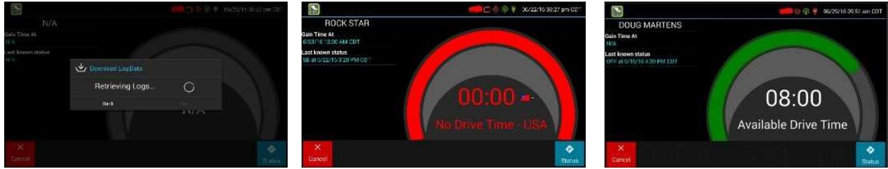
When a message is received that logs are received or up to date, click **OK** to view the last recorded duty status and current driving time left. The device will indicate driving time left to be previewed before completing the sign in process.
