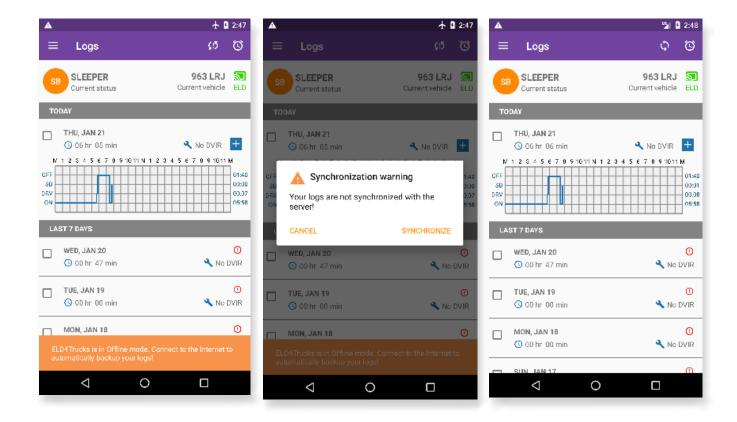
1. When this occurs, an "Un-sync" status icon will appear instead of "Sync" icon. This indicates a failure to synchronize with the server. This icon will also appear when there is no internet connection and the device has records that need to be sent to the server.
